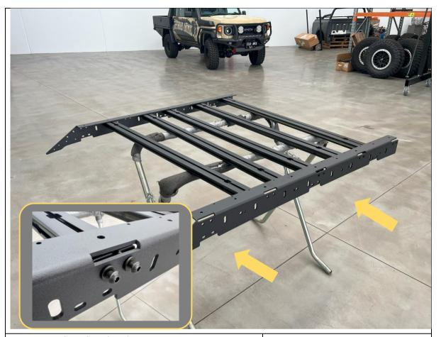
3. Fit the side rail to the extrusion,
